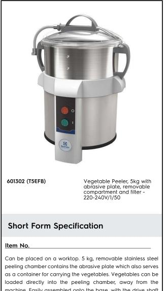
machine. Easily assembled onto the base, with the drive shaft fitting into the centre of the plate. The transparent cover closes the cylinder during the peeling operations. Timer pre-set to 3 minutes. Peeling speed: 305 rpm. Removable water inlet, on the cover, designed to serve as a spray for cleaning the machine. The electronic controls and the motor of the peeler have IP55 protection. Optional drying basket.
